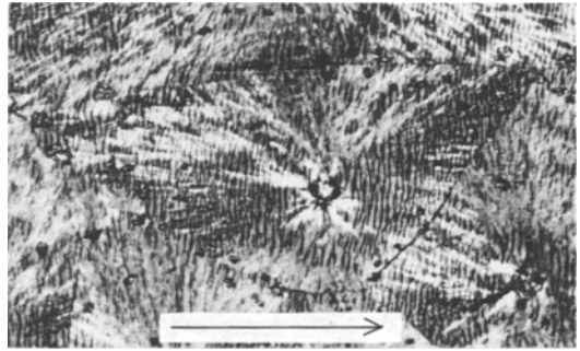
Figure. 15 Micrograph of a two dimensional POM spherulite that has been extended by 10% on a 'Mylar' substrate. The arrow shows the direction of extension.
